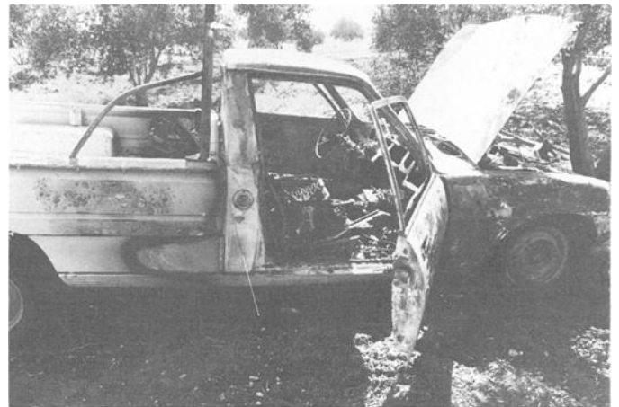
FIG. 1—The front passenger compartment of the van was found burned.
